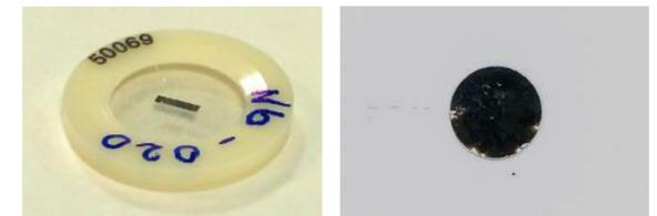
Figure 3: Nb dosimeter (left) and Rh dosimeter (right)
