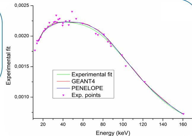
Figure 2: Efficiency calibration curve with Monte Carlo method
