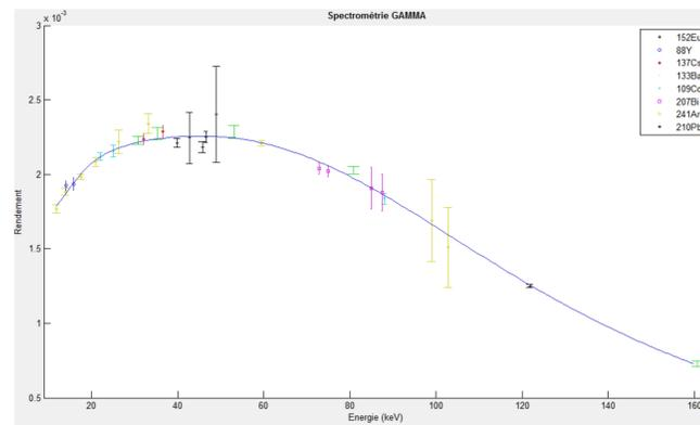
Figure 1: Experimental efficiency calibration: experimental values and fitted curve
