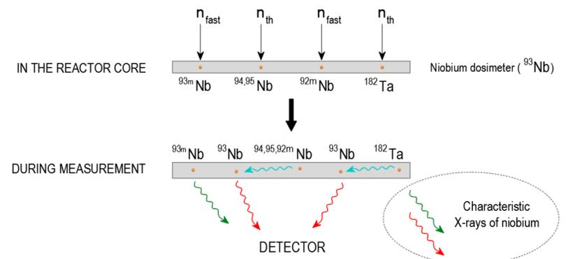
Figure 4: Self-fluorescence in niobium dosimeters
