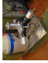
System using TDCR scintillation detection system in the beta counting channel
