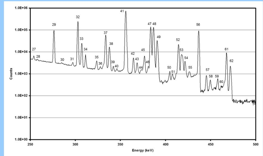
Spectrum of a  $^{133}\text{Ba}$  point source measured in high efficiency conditions
