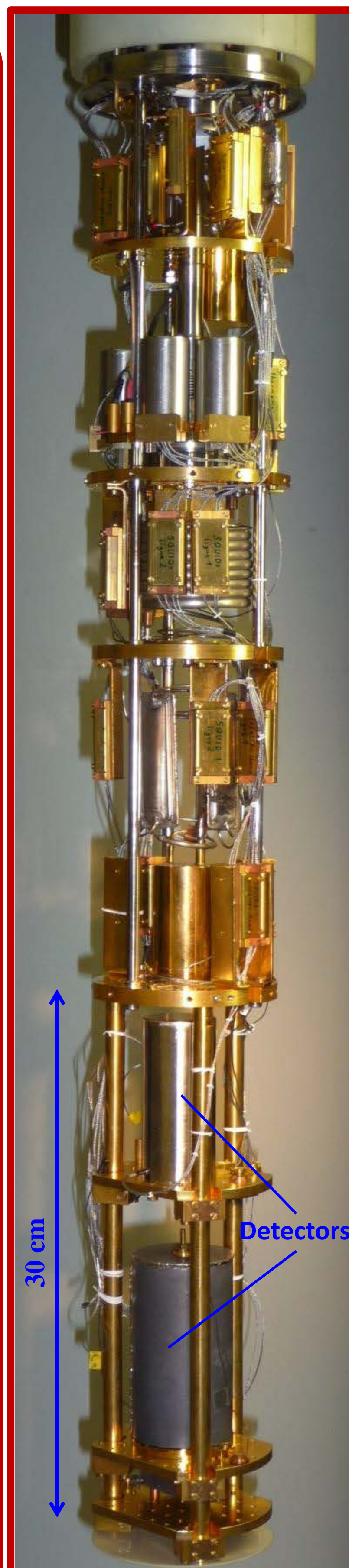
Dilution refrigerator at LNHB (Base temperature < 10 mK)
