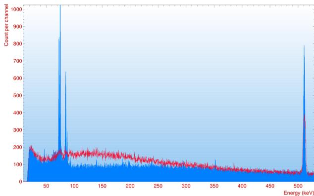
If it is thick enough, the internal copper shielding removes all lead X-rays. However, as shown on the pictures, it should only be used if the veto system correctly eliminates the 511-keV contribution:
